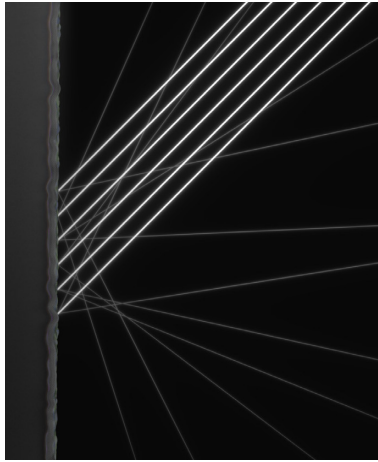
Light scattering on nano-texture cover glass
